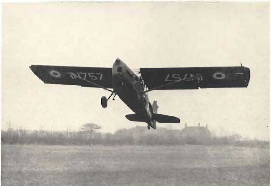
With flaps set at 'Take-off', and ailerons drooped, an Indian Air Force Mk. 9 climbs away at a characteristic angle. The Mk. 9 can be lifted off the ground in a three-point attitude and will continue to climb without any tendency to sink back or stall.
