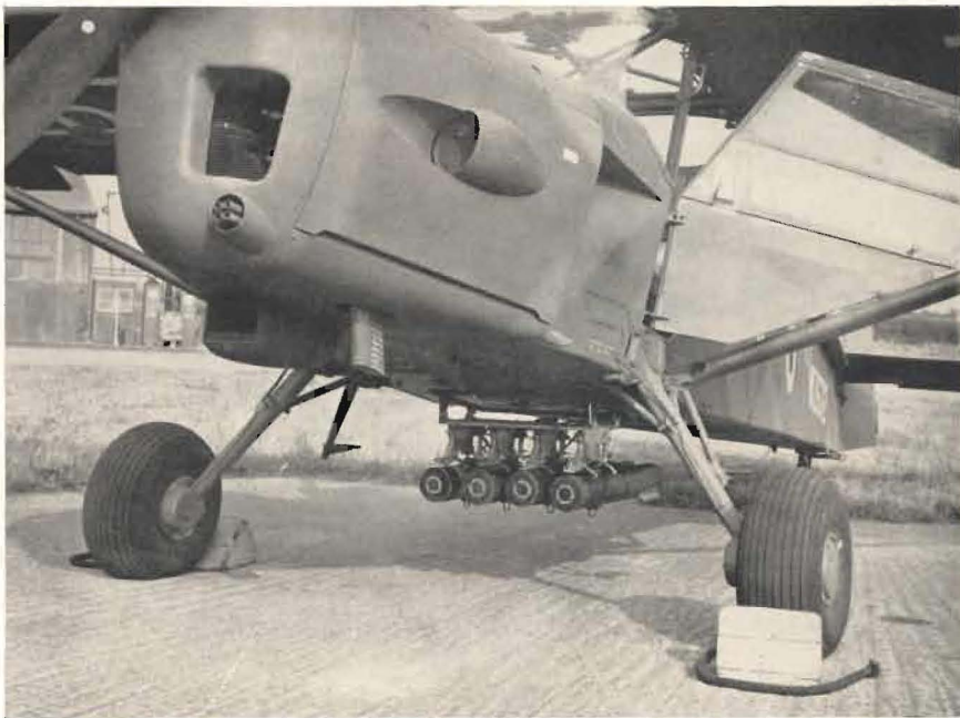
To widen its operational scope, trials have been carried out with an Auster A.O.P. Mk. 9 fitted with a light series bomb carrier. It is seen here with four 4" flares in position.
